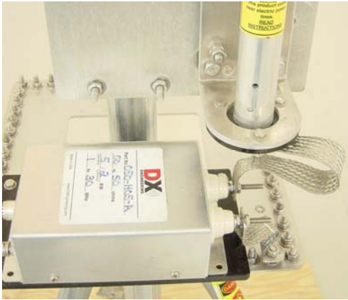
Figure 1 Insulated Balun System for use with Hustler Antenna and Radial Plate. The braid is sized for use with the Tilt-Base and Radial Plate.
